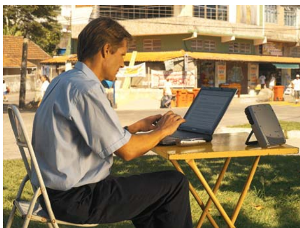
Figure 4 Example of BGAN Terminal usage
